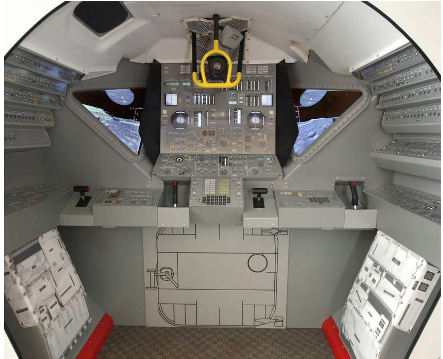
*The Lunar Landing Simulator by Historic Space Systems installed at the Joliet Area Historical Museum in Joliet, IL. Features include accurately modeled window frames, glare shields, molded fiberglass ceiling, Alignment Optical Telescope and guard, storage compartments, consoles, and a hatch representation.*
