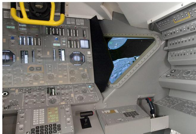
The Lunar Module Pilot's panel is modified to include the gauges needed for an independent landing.
