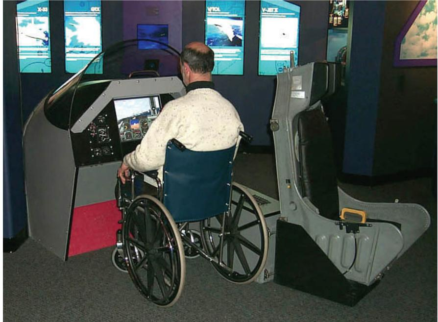
*This Aircraft Simulator by Historic Space Systems is installed at the Visitor Center of the NASA Glenn Research Center in Cleveland, Ohio. The ejection seat rotates out for wheelchair access, or locks firmly in place for ordinary use. NASA supplied the ejection seat and control panel gauges. Historic Space Systems integrated these items into the exhibit. (Pictured with David Lowenfeld of NASA Glenn.)*
