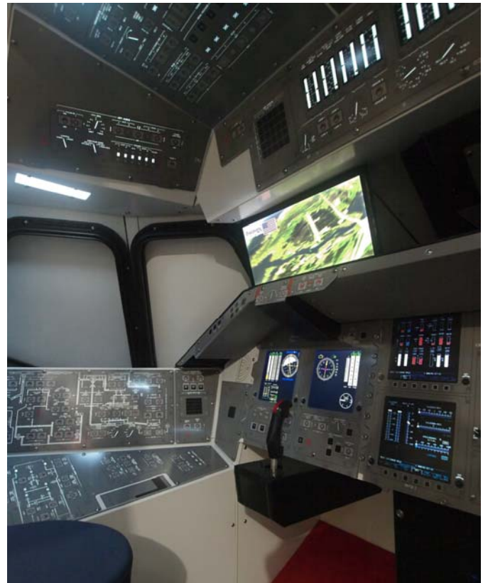
The Commander's side of the Space Shuttle Landing Simulator. The HD monitor at top displays the forward window view. A single monitor in the console displays the simulated flight gauges as if they were on two monitors. (The two monitors at right are static graphic displays.) Control panels are backlit, similar to the actual panels, using long-life LED lighting. Window frames detail the features of the actual frames for an enhanced feeling of “being there.” (National Museum of the USAF simulator shown.)
