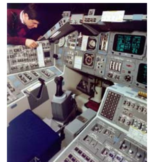
The Commander's side of the Space Shuttle Landing Simulator. The HD monitor at top displays the forward window view. A single monitor in the console displays the simulated flight gauges as if they were on two monitors. (The two monitors at right are static graphic displays.) Control panels are backlit, similar to the actual panels, using long-life LED lighting. Window frames detail the features of the actual frames for an enhanced feeling of “being there.” (National Museum of the USAF simulator shown.)
